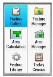
GPSMAP 64sc SiteSurvey comes with built-in Garmin unique custom attribute collection capabilities, supports computer-based Garmin SiteSurvey PC software. Before data collection, users can pre-define targeted features and their attributes before getting in the field through SiteSurvey computer based tool and import to GPSMAP 64sc SiteSurvey device. After field data collection, users can export the collected data to SiteSurvey for post-processing.
